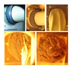
The basis for the fire protection product is the intumescent substrate brought onto the layer on both sides.
