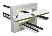
3. Seal remaining openings tightly with mineral wool and/or close with PYRO-SAFE® FLAMMOTECT-A.
